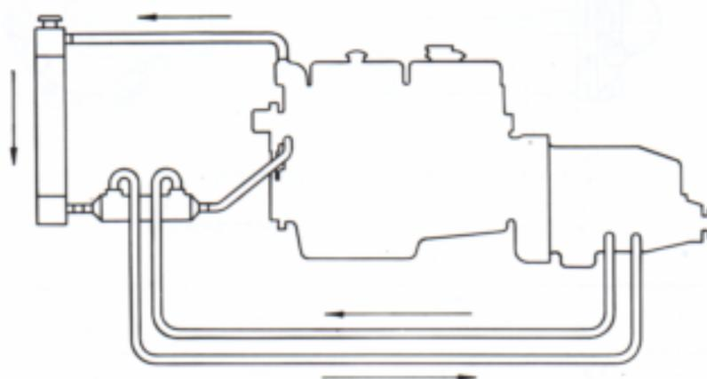
Installation of an oil cooler in an engine water circuit.
