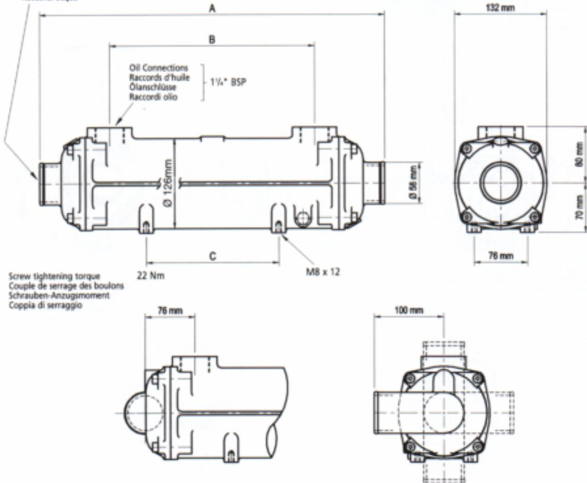
Screw tightening torque
